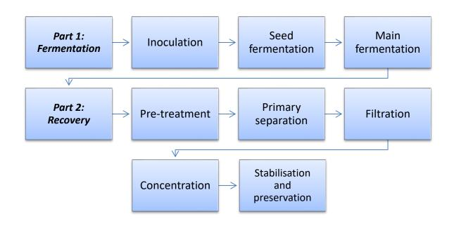
Figure 2: Manufacturing process for triacylglycerol lipase preparation
